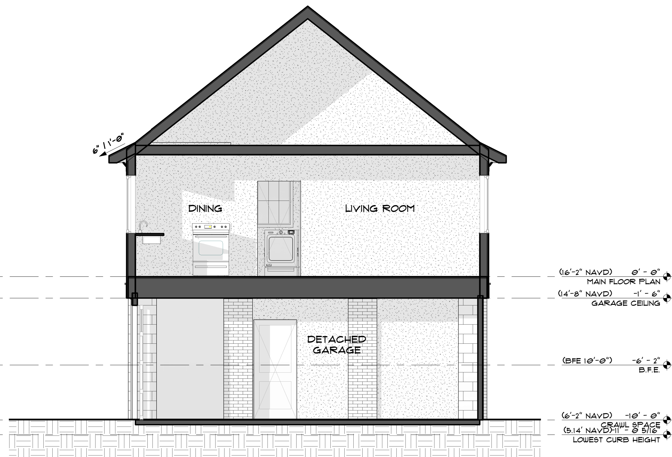
GARAGE BUILDING SECTION @ LIVING/KITCHEN SCALE: 1/4" = 1'-0" ③
